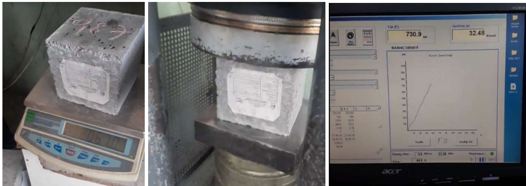
Figure 10.5.1.3.1 – Compression test on a cubic C30/37 concrete sample
