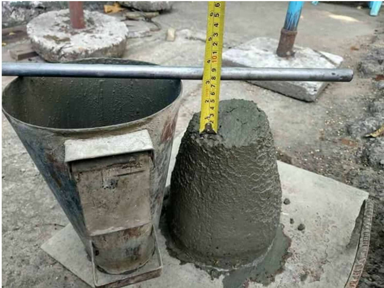
Figure 10.5.1.2.1 - Concrete Slump Test [13]
