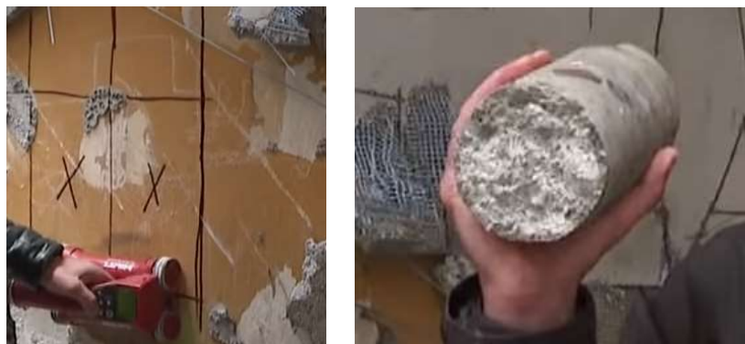
Figure 11.5.3.3.1 – Core Testing Preparation and the Core Extracted
