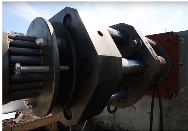
Figure 3.2.6.1 – (Left) Eugene Freyssinet [12] and (Right) Modern Freyssinet post-tensioning equipment from construction of North Marmara Highway, Istanbul, Turkey (Feb 18, 2016)
