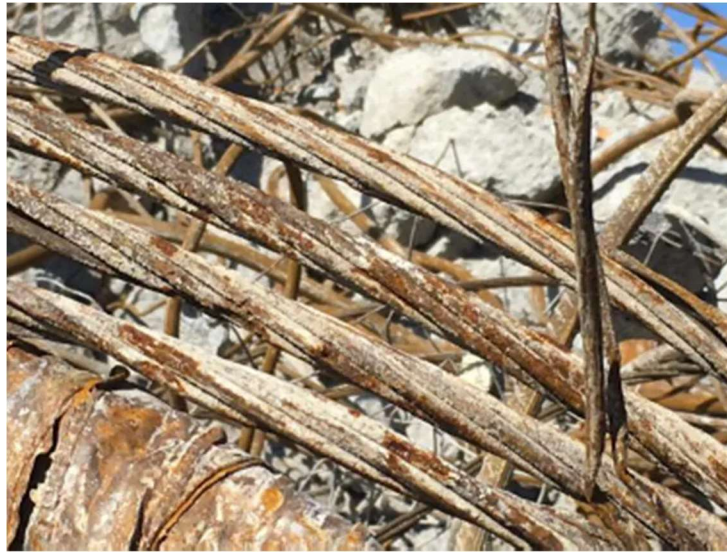
Figure 2.4.3.3 - Photo of corroded steel and prestressing steel of the collapsed section [17]
