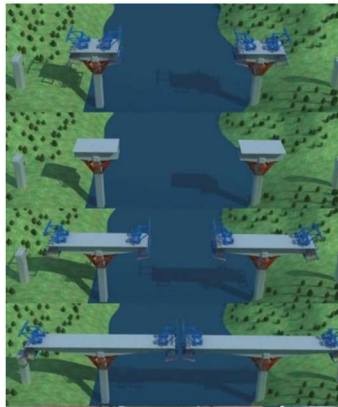
Figure 6.4.2.2 - Balanced Cantilever Segment Approach
