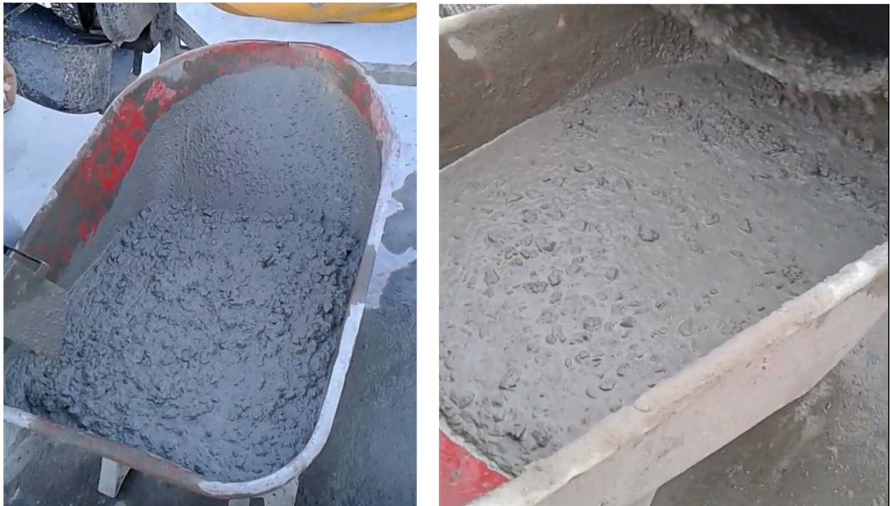
Figure 3.2.4.2 – (Left): C30 Concrete: 310 kg Cement, 1.2% Grace Ex 3282, 0.03% Daravair1000 (Air-entraining admixture), 7.2% Air and (Right): C40 Concrete: 370 kg Cement, 1.1% Grace Ex 3282, 0.03% Daravair1000 (Air-entraining admixture), 7.2% Air
