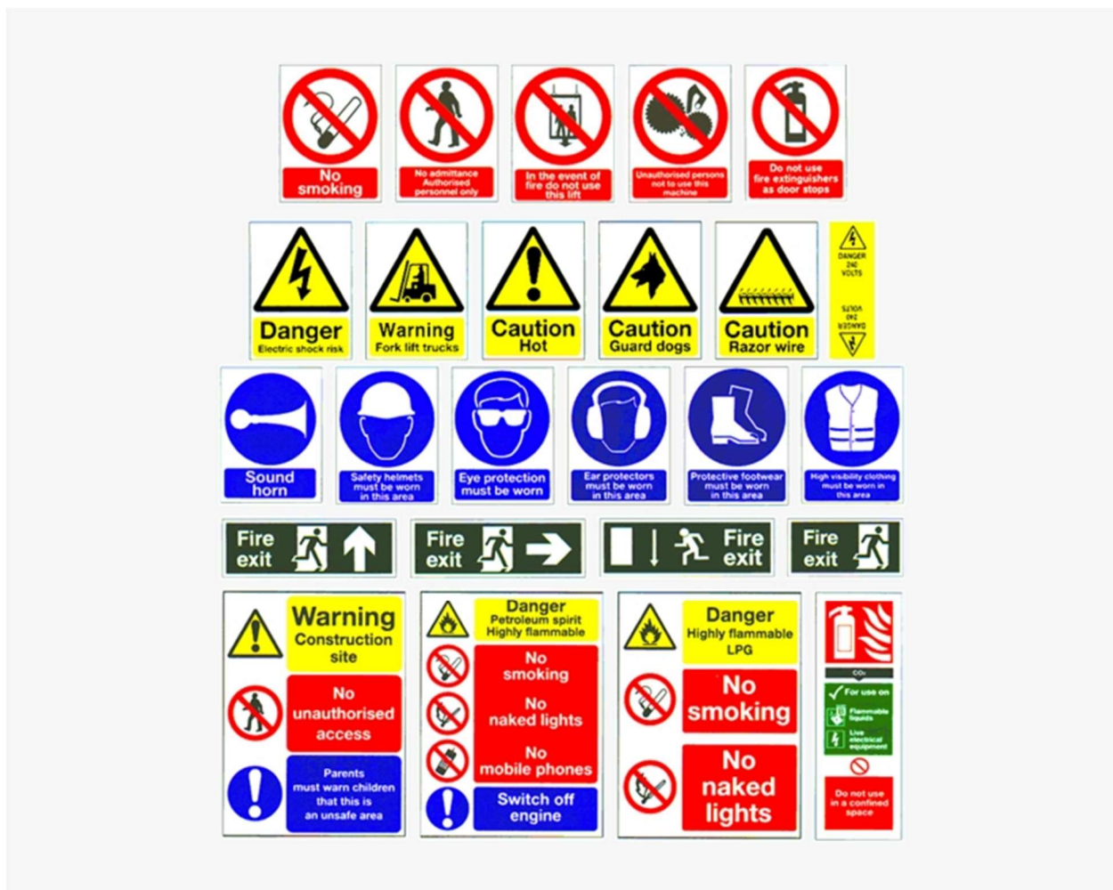
Figure 10.2.4.1 - Example of Common Construction Safety Signs [6]
